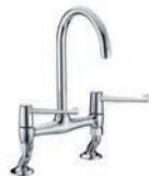
Bridge Sink Mixer Height 390mm Spout projection 175mm 6" Levers Dual flow prevents hot water entering the mains supply
