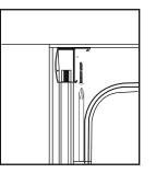
5 - Reposition the assembly and fix the wall channels to the wall using 8 x ST4x30 long screws (4 per channel).
