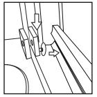
9 - Once the door is ready it needs to be hung in the enclosure, start by lifting the door up and guiding the top support wheels into the top horizontal profile, then using the quick release mechanism on the bottom wheels guide them into the bottom horizontal profile as shown.
