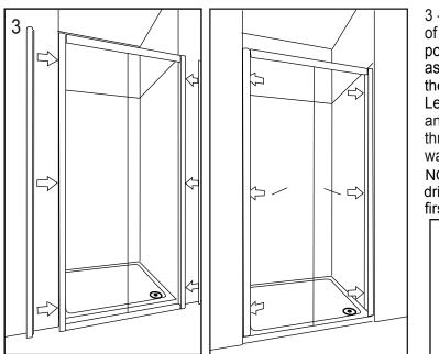
3 - Push the wall channels onto the edges of the assembly as illustrated and then position the assembly onto the shower tray as shown (roughly 10mm from the front of the tray).
