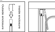
4 - Remove the assembly and drill the marked points using a 6mm masonry drill bit, once this is done insert 8 x wall plugs into the holes.
