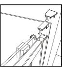
10 - Once you are happy that the installation is correct and that the door is running smoothly, push the cover caps onto the edges and tops of the wall channel as shown, (smaller top cap first followed by the larger wall channel top cap and then the wall channels snap on cover) then silicone the outside of the enclosure where the metal profiles meet the wall and the tray.
