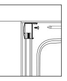
6 - Whilst using the available play to ensure that the assembly is central between the wall channels and held against the shower tray at the bottom fix the assembly to the wall channels by drilling through the pre drilled holes in the wall channels into the profiles using a 2.75mm metal drill bit. Then secure using 8xST3.5x10 short Screws (4 per wall channel).
