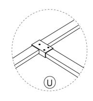
T-piece connector for end panel support bar
