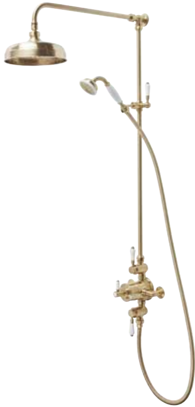
Keswick dual function shower system with rigid riser kit & overhead shower • Brushed brass thermostatic sequential shower valve • Height adjustable rigid riser rail with separate flow control to overhead shower and handset • Overall system height 1237mm, rigid riser rail can be cut to height • 200mm brushed brass shower head • Single function brushed brass shower handset • Brushed brass shower hose • Min pressure 0.5bar
