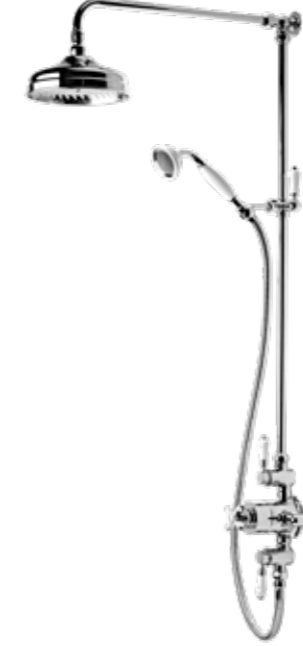
Wessex dual function shower system with rigid riser kit & overhead shower • Thermostatic sequential shower valve • Height adjustable rigid riser rail with separate flow control to overhead shower and handset • Overall system height 1237mm, rigid riser rail can be cut to height • 200mm brass shower head • Brass shower hose Min pressure 0.5bar
